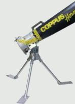
JECTAIR TRIPOD For stationary, long-term use; rotates 360 degrees for precise direction of air-flow and accommodates 3-HP and 6-HP Jectair sizes. Installs quickly and easily with two quick-release clamps. Large feet provide stability during operation, and spring-loaded legs fold up for easy transport and storage.
