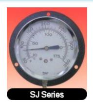
The Model SJ dial thermometer withstands vibrating conditions to give accurate temperature indication. Its liquid actuated temperature sensing system utilizes a spiral wound Bourdon tube that absorbs shock. Steady operation results, which combines with the 3 ½" dial size for ease of reading. The Model SJ is available in a variety of case styles and with a selection of temperature measurement ranges.
